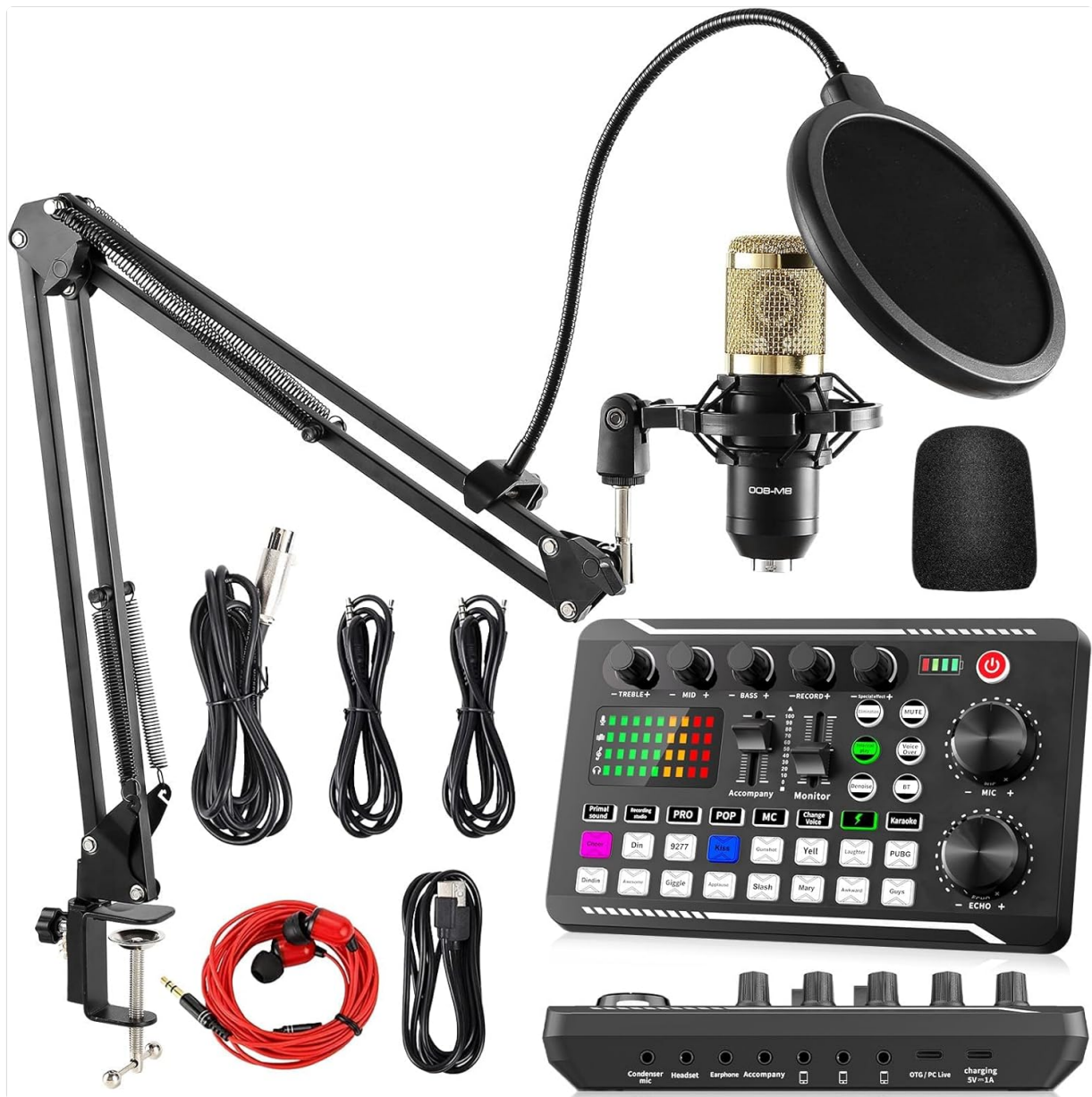
Image 4: The BM800 Condenser Microphone, shown with its shock mount, pop filter, and anti-wind foam cap.
