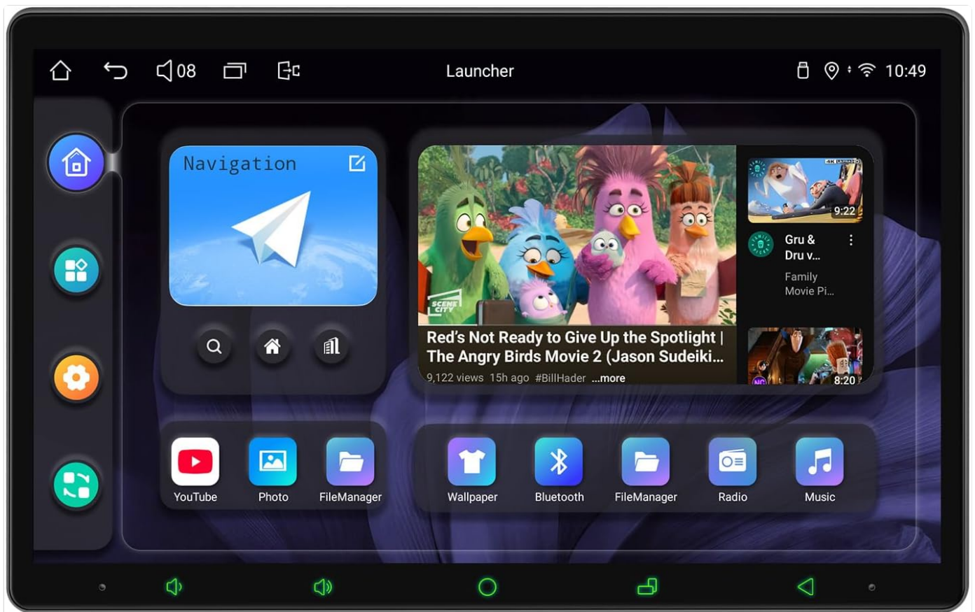
Figure 4.1: The main user interface of the Joying 11.6 Inch Double Din Car Stereo, displaying navigation, media, and various application shortcuts.
