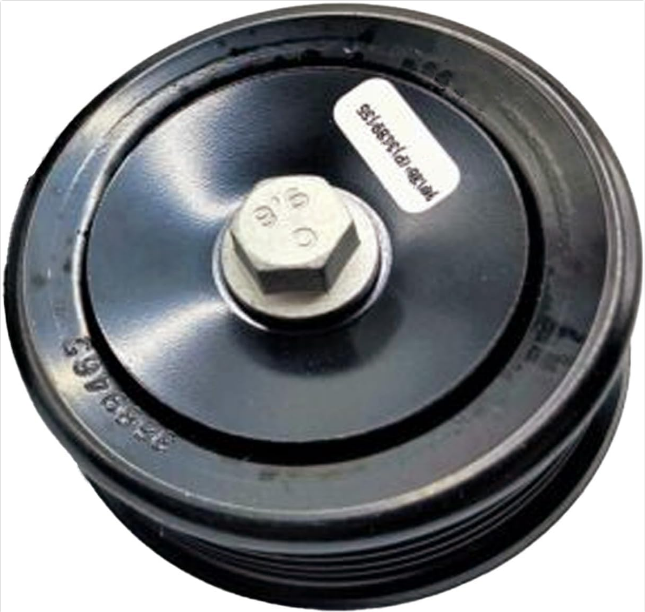
Image 1.3: Detailed view of the XYohykai Idler Pulley, highlighting the bearing and a label with part number '3689465', indicating the specific model.
