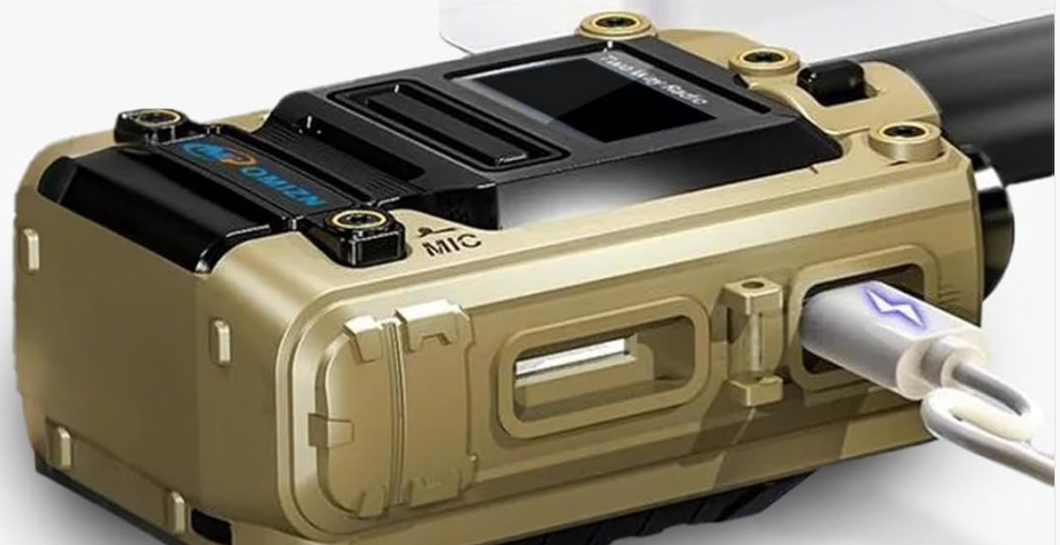
Image 4.1: The OMIZN M8 radio connected to a power adapter via its Type-C port for charging. Various charging methods are depicted, including power bank, car, PC, and Type-C wall charging.
