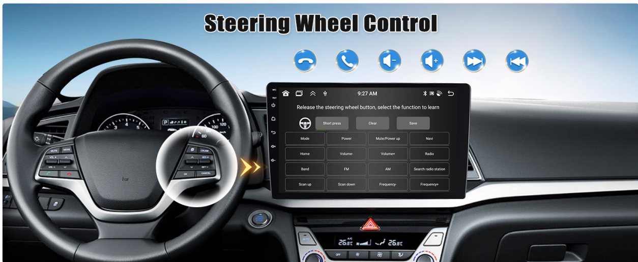
Figure 3.14: Steering Wheel Control. This image shows the car stereo's interface for programming steering wheel controls, allowing users to assign functions like volume adjustment, track skipping, and call answering to their vehicle's existing buttons.
