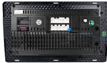
Figure 2.3: Backup Camera and Canbus Connection Diagram. This diagram illustrates the wiring for the backup camera, showing connections for the red cable to the positive reversing light, the black cable to the negative reversing light, and emphasizing the white plug connection to the main unit for Bluetooth and WiFi functionality.
