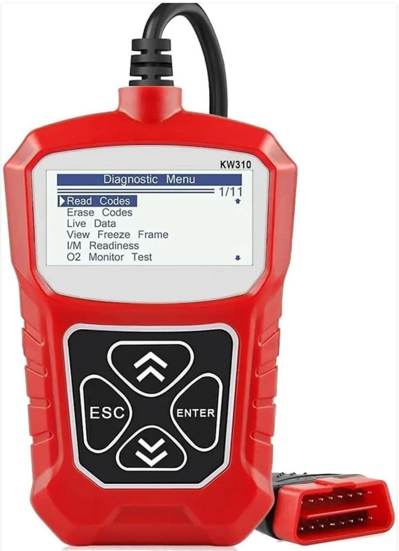
Figure 1.1: The XAUCY KW310 Car Scanner with its diagnostic menu visible, showing options like Read Codes, Erase Codes, and Live Data.
