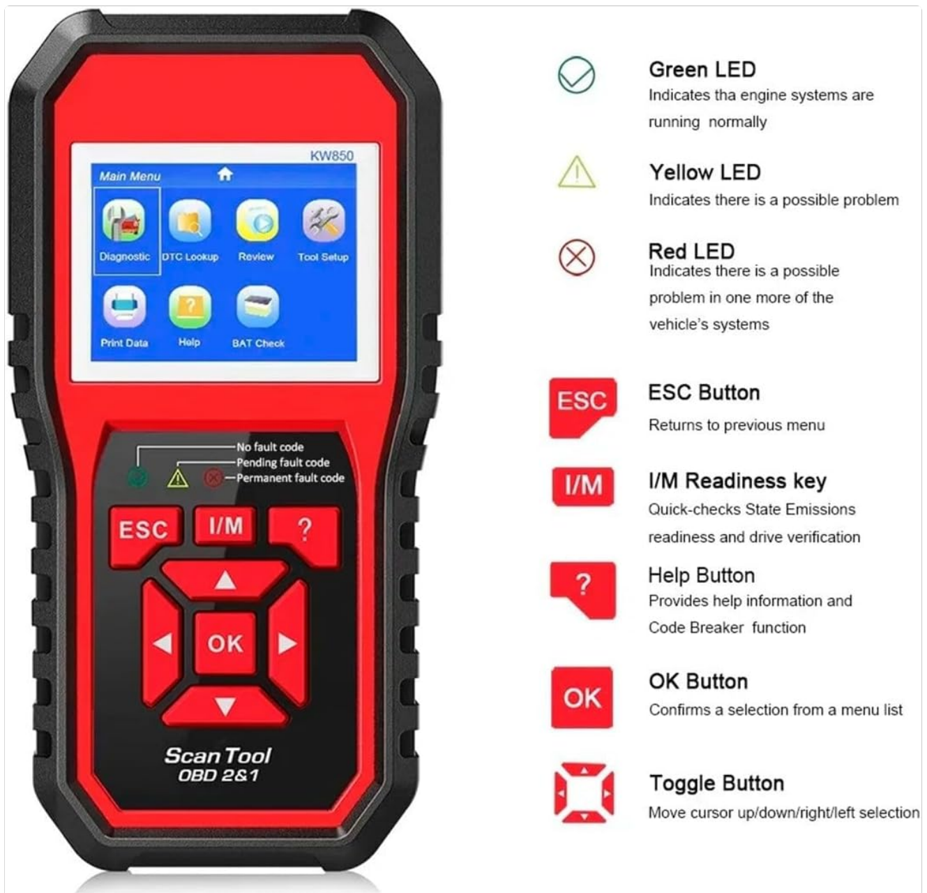
Image 5.1: The KW850 scanner's LED indicators: Green for normal engine systems, Yellow for a possible problem, and Red for a definite problem in one or more vehicle systems.
