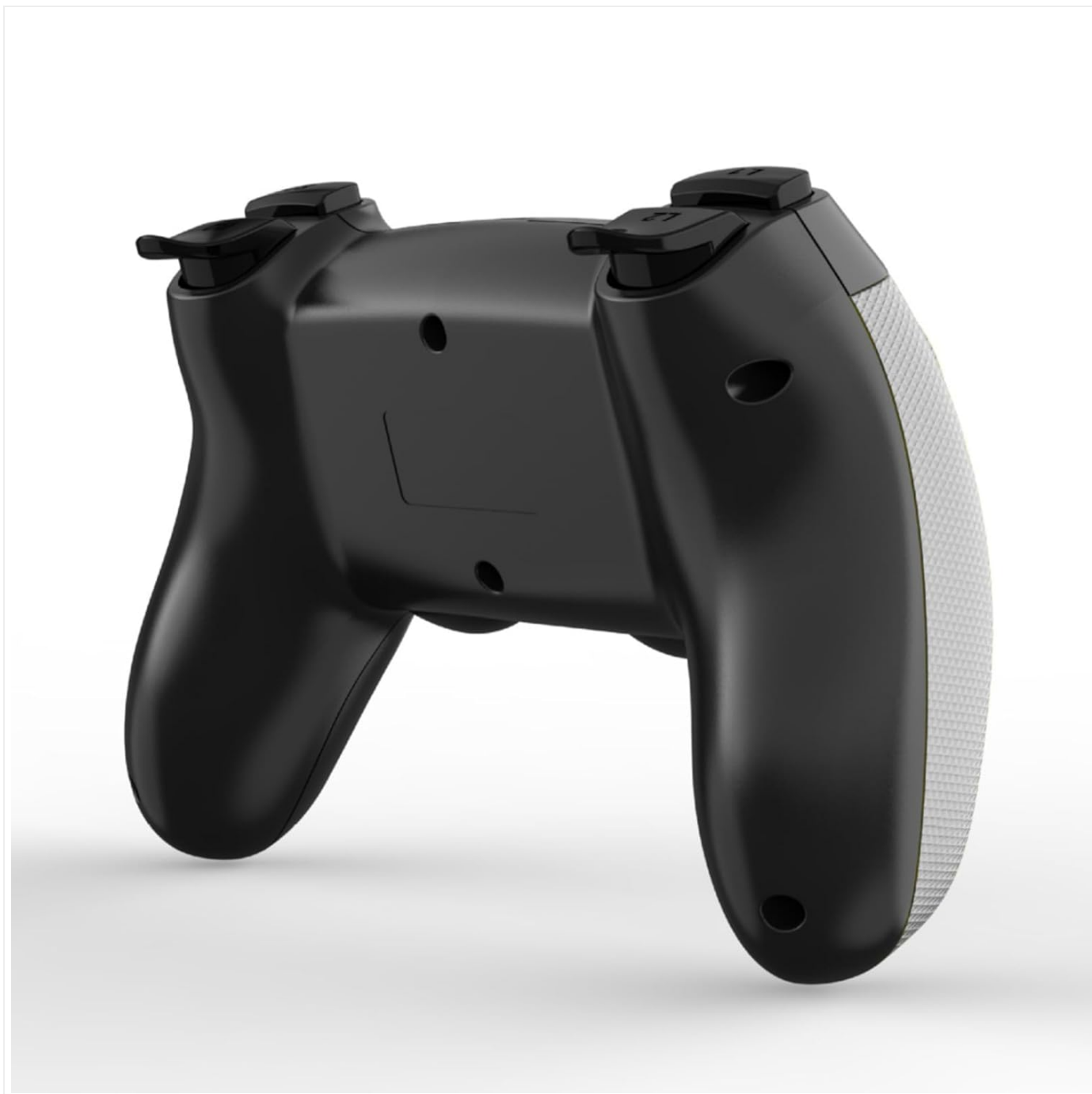
Image: Rear view of the gamepad, indicating the location of the battery compartment.
