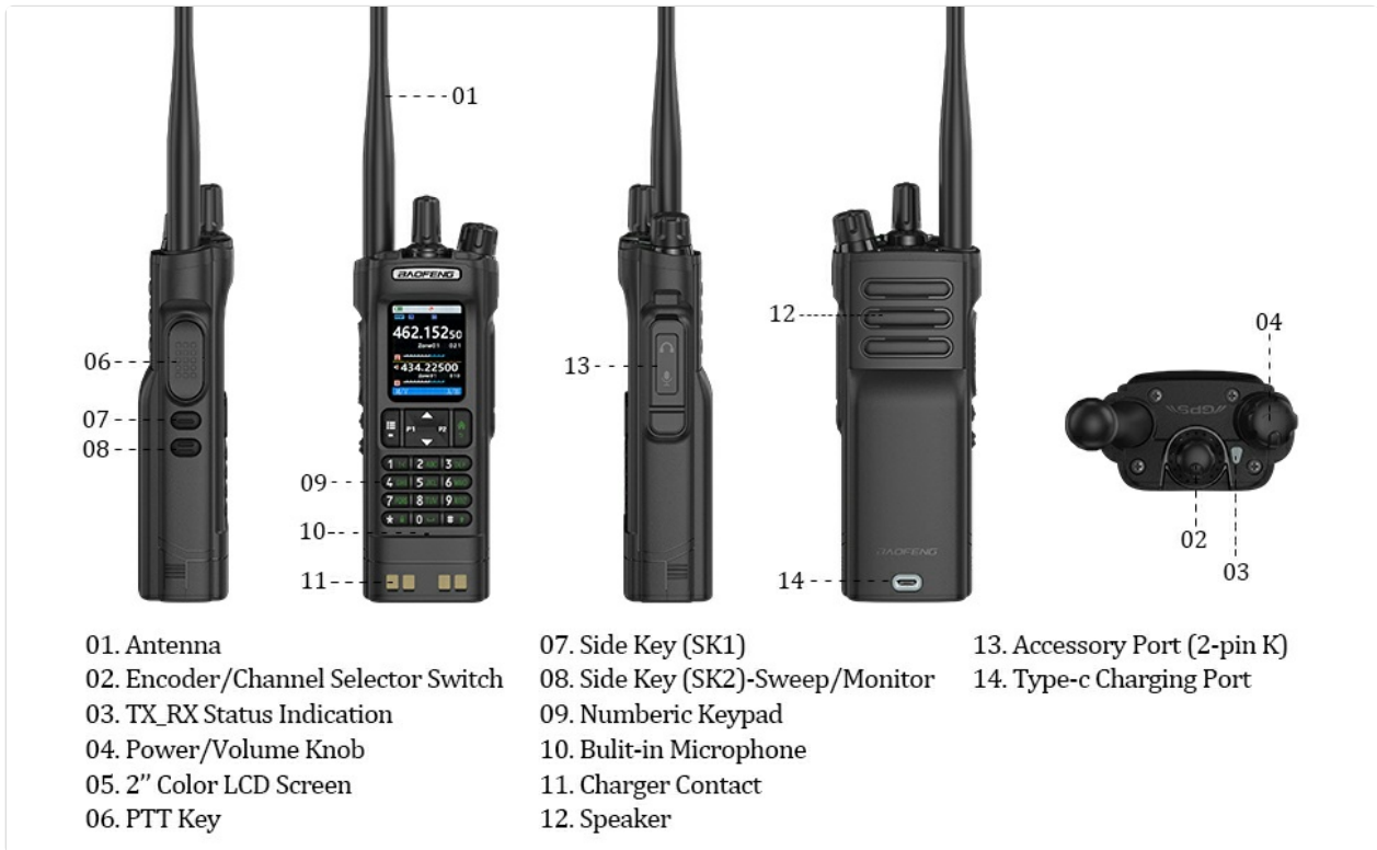
Figure 4.1: BAOFENG UV-32 Radio Component Diagram
