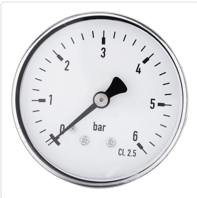
Figure 3.2: Front view of the TS-60 dial, clearly showing the 0-6 bar scale and 'CL. 2.5' accuracy class.
