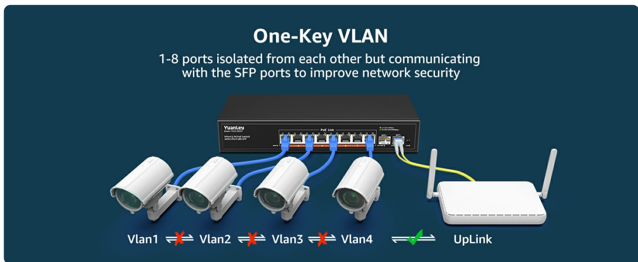
Image: A visual explanation of the One-Key VLAN feature, demonstrating how ports are isolated while maintaining uplink connectivity.
