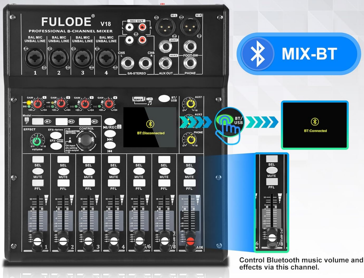
Figure 5: Illustration of the built-in Bluetooth feature for wireless audio streaming.
