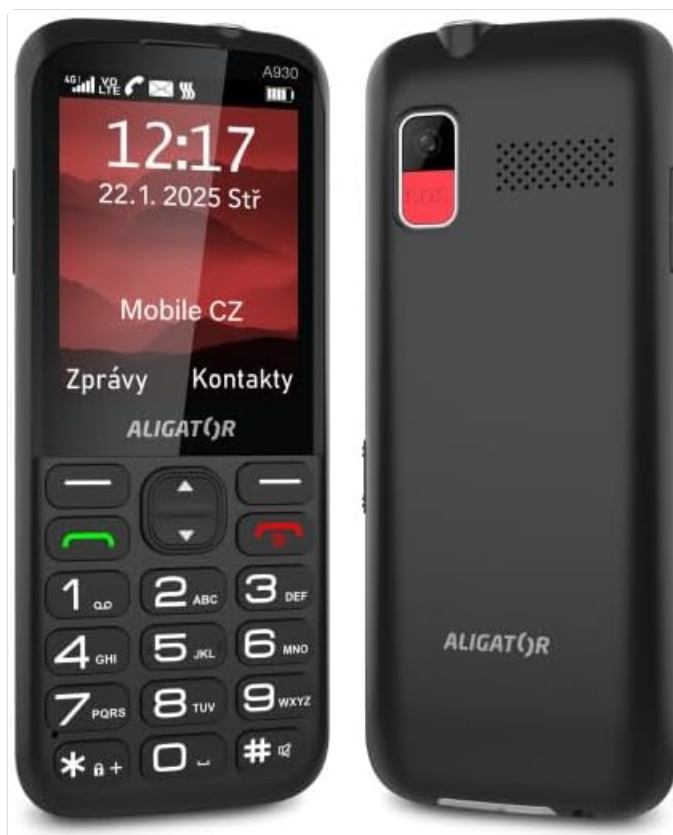
Figure 5.1: Rear view of the ALIGATOR AZA930B, showing the prominent red SOS button and the speaker grille for clear audio.
