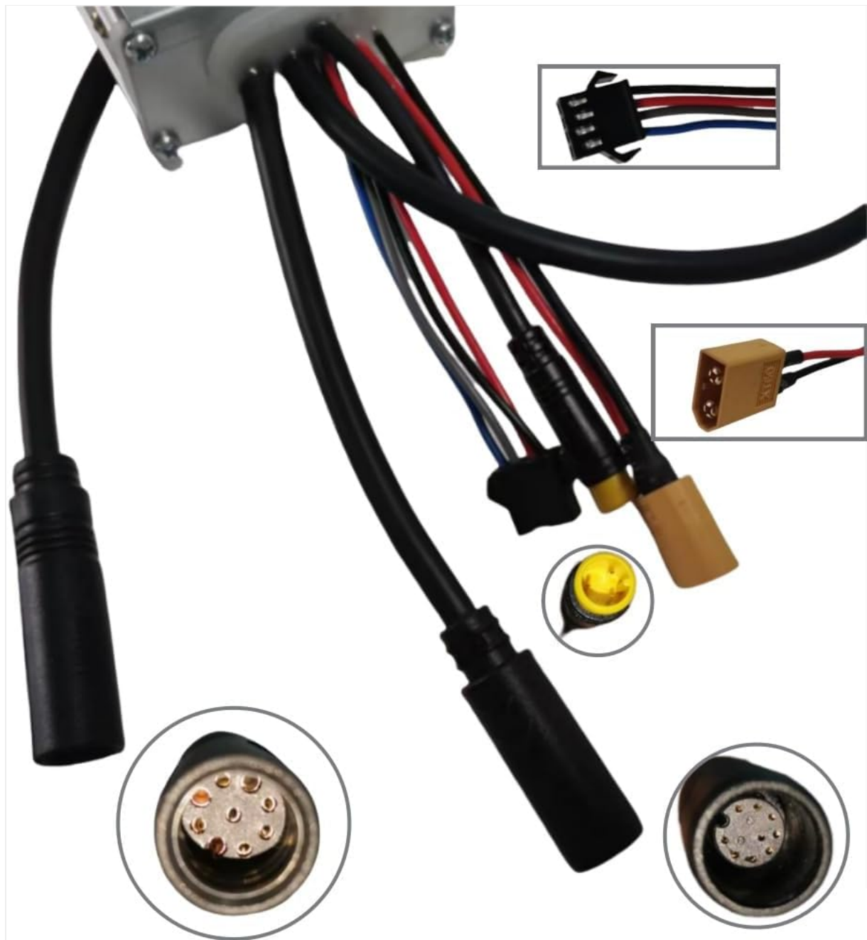
Figure 4: Detailed view of the various connectors and wiring harnesses extending from the controller, including power, motor, and display connections.
