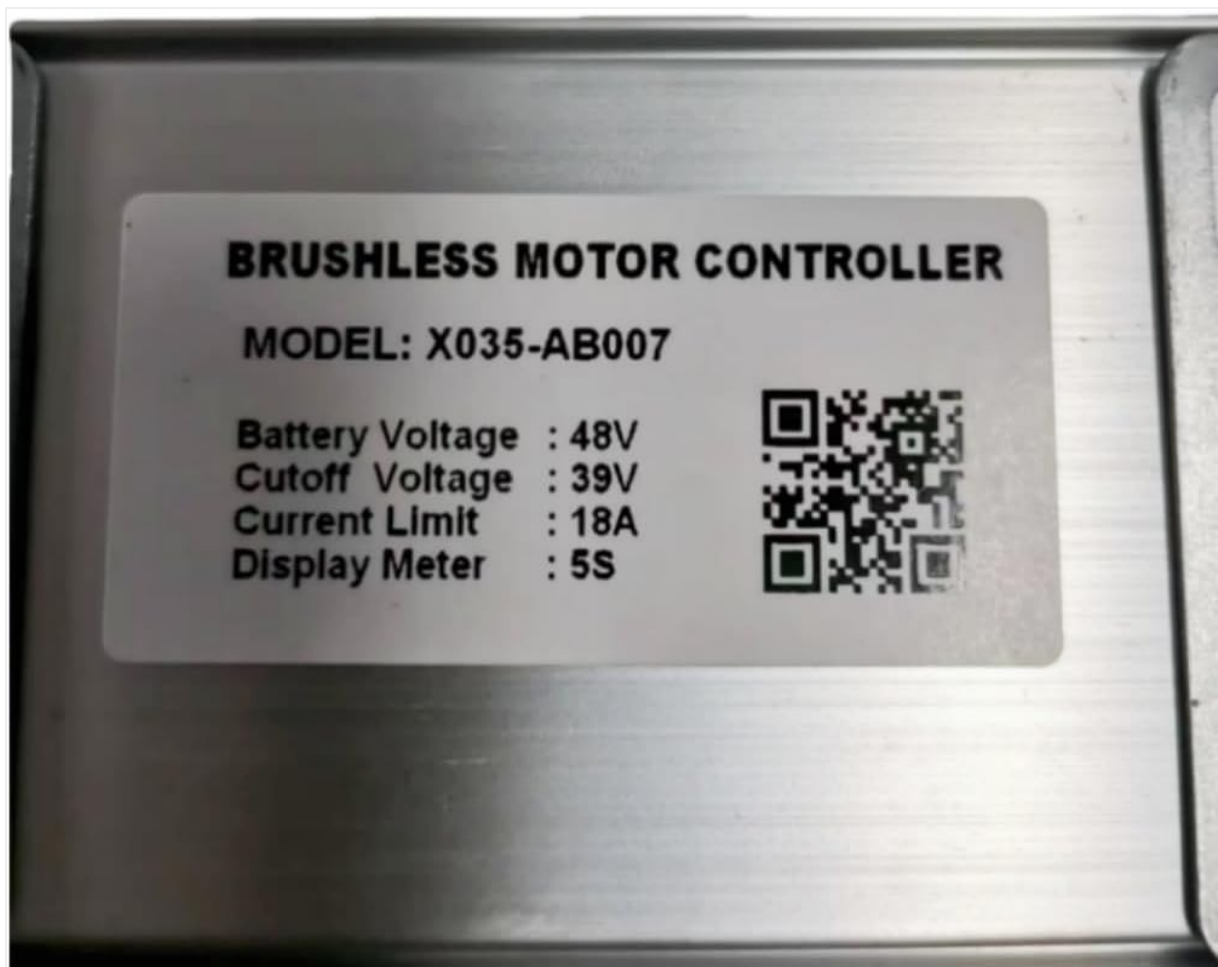
Figure 2: Close-up view of the controller's identification label, showing model number X035-AB007, Battery Voltage (48V), Cutoff Voltage (39V), Current Limit (18A), and Display Meter (5S).
