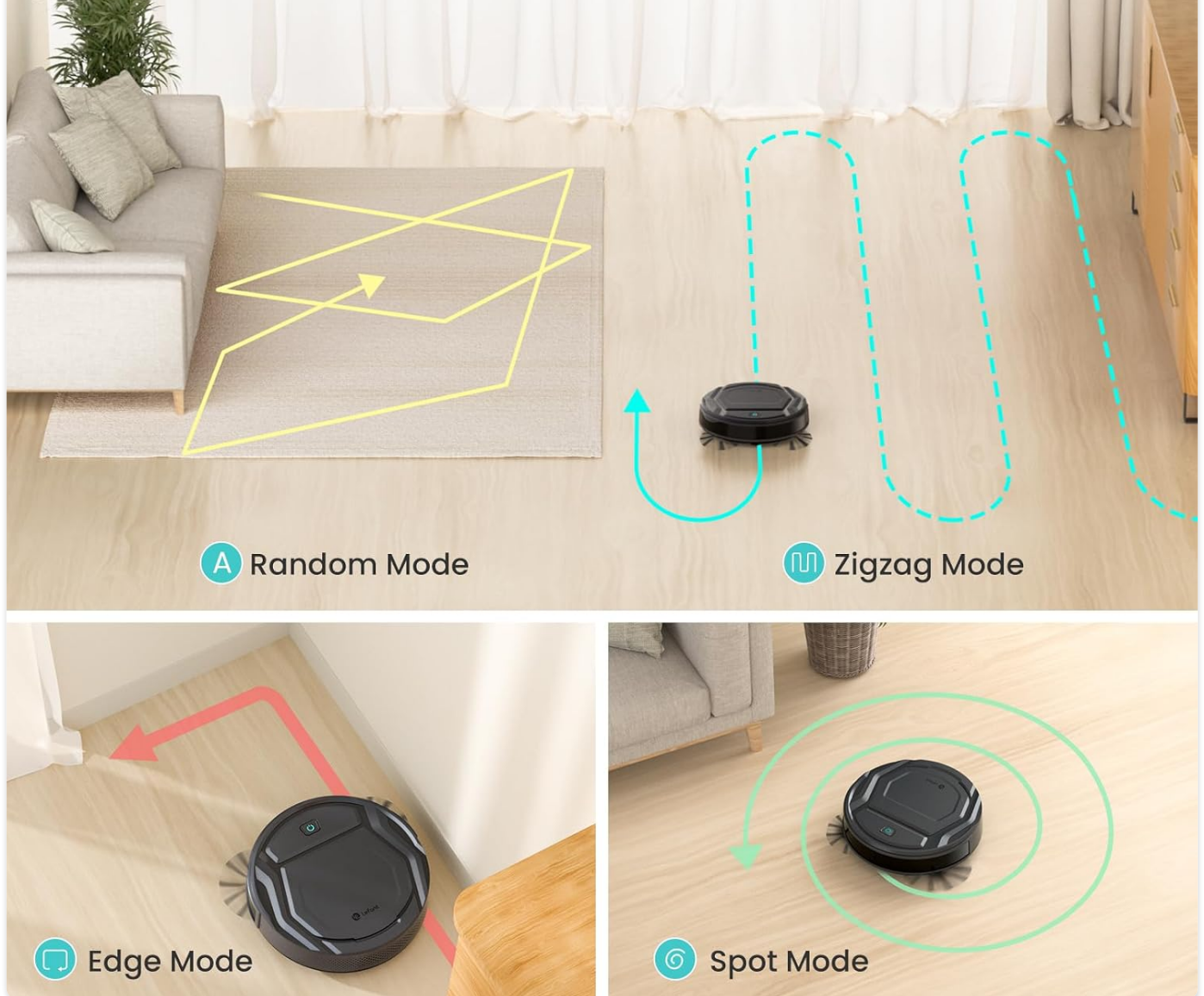
Figure 3.1: The M210P supports various cleaning modes including Random, Zigzag, Edge, and Spot to meet diverse cleaning requirements.
