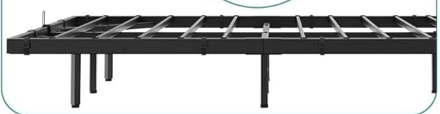
Image 4.1: Important installation method for the middle T-shaped support slat. Ensure it is perpendicular to the side rails and level with their top edge to prevent frame bulging.
