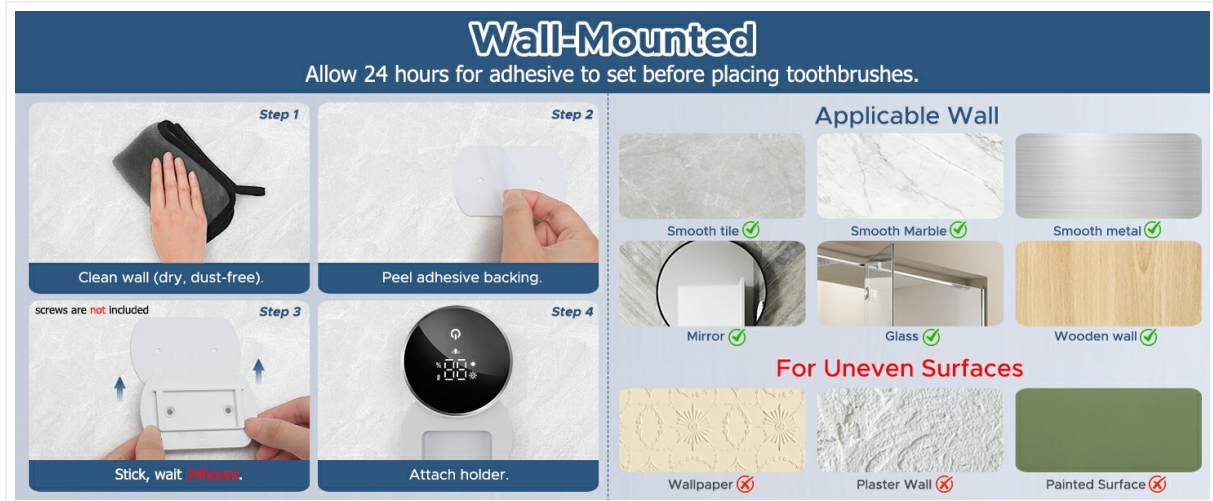
Image 3.1: Visual guide for wall mounting and compatible wall types.
