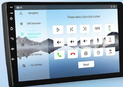
Image 4.4: GPS Navigation, WiFi, Backup Camera, and Steering Wheel Control features.
