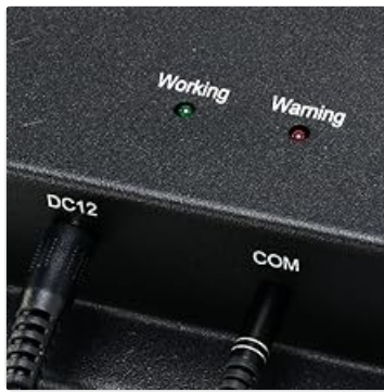
Figure 2.4: Power and Control Ports.
