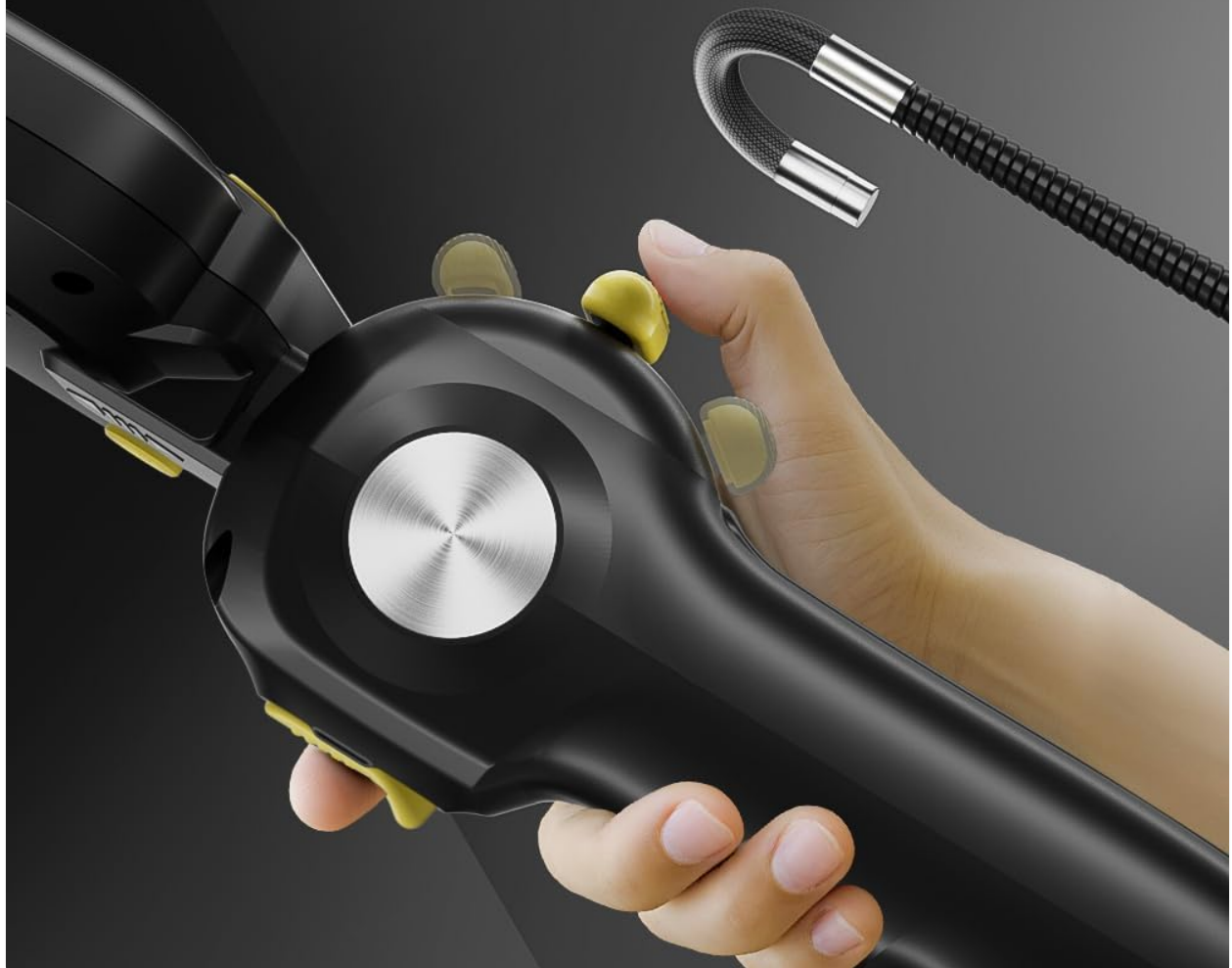
Figure 3.3: The device features a one-handed operation design, where the thumb controls the push-pull rods for probe articulation, and the index finger operates the photo capture button.
