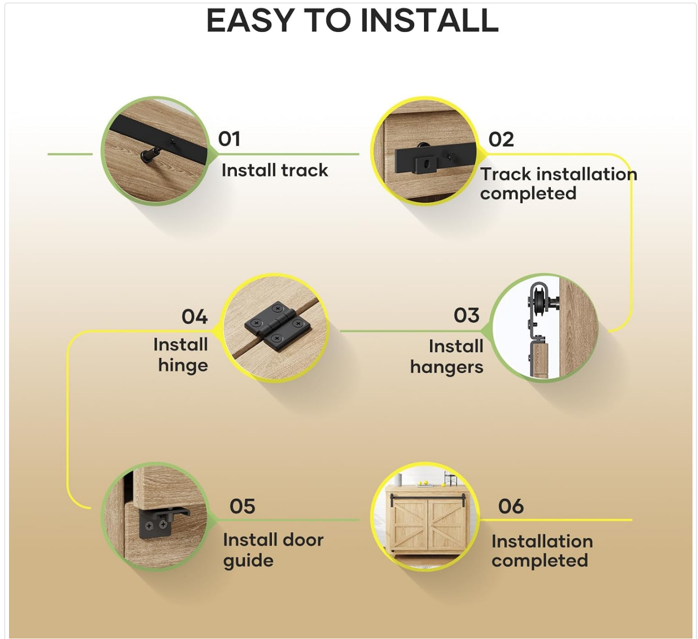
Image 5.1: Visual guide to the installation steps.
