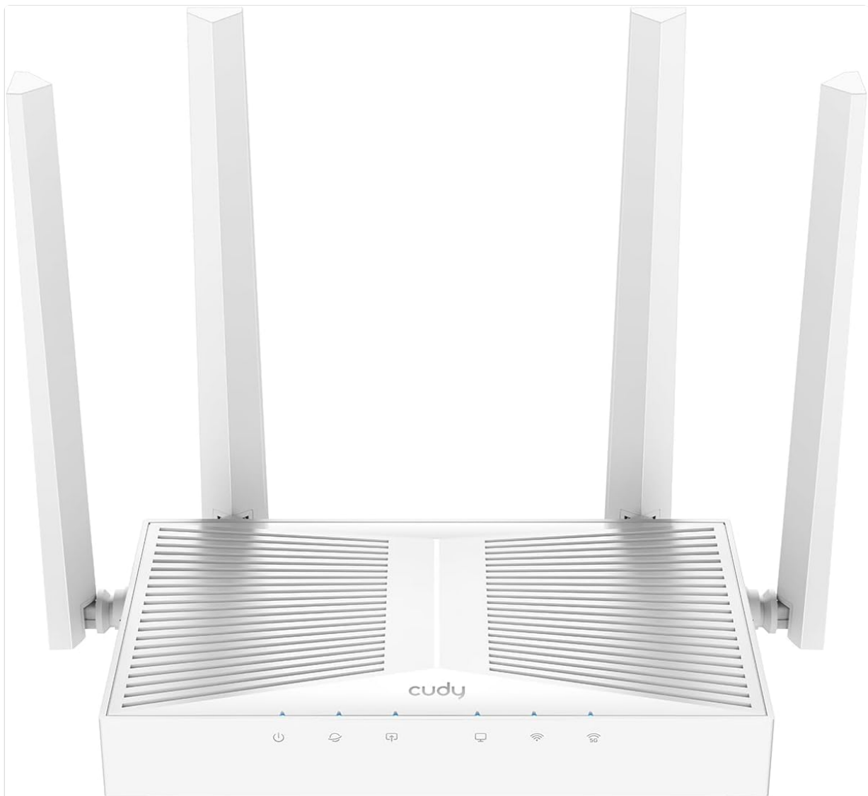
Image 3.1: Front view of the Cudy WR3000E router, showing its four external antennas and LED indicators.
