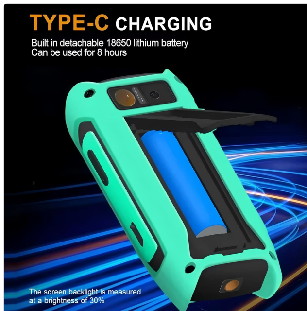
Figure 4.1: Illustration of the Type-C charging port and the detachable 18650 lithium battery compartment on the ET14C.
