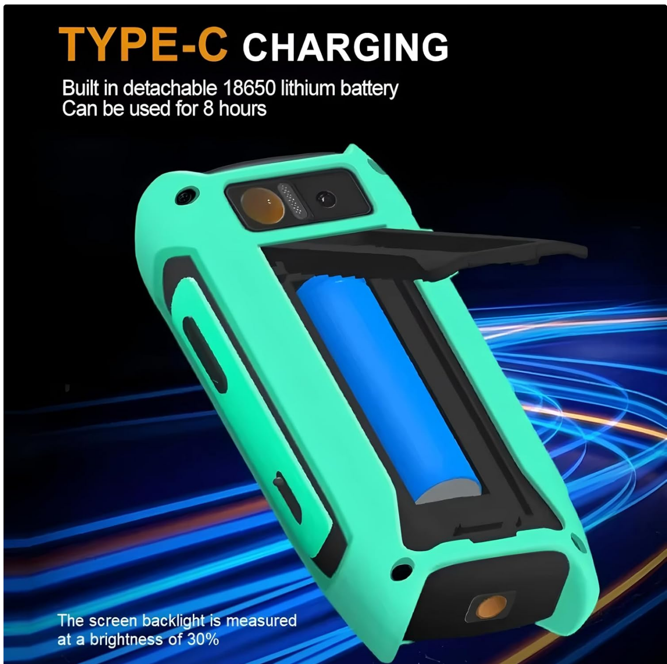
Figure 4: Battery installation and Type-C charging port.
