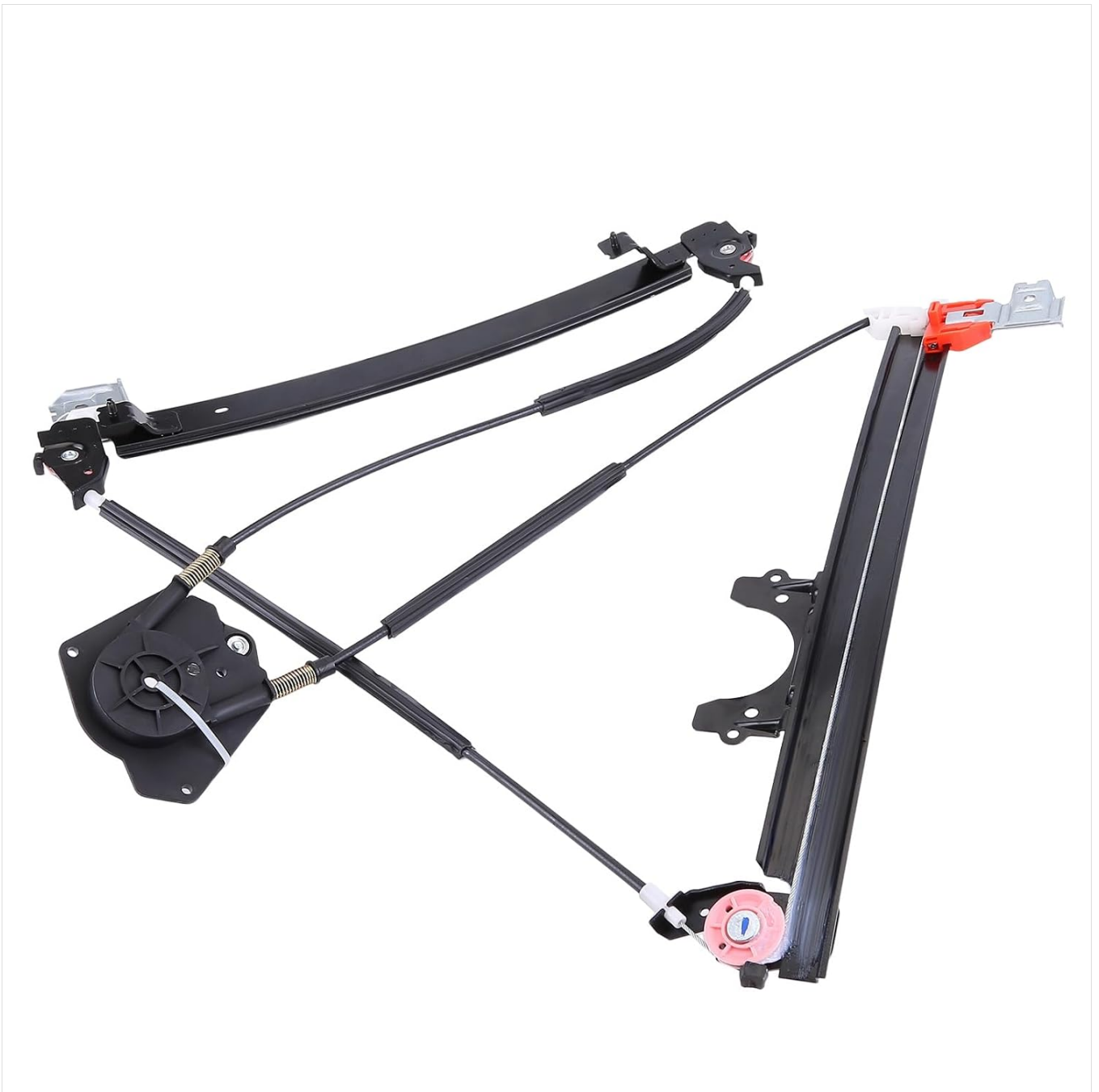
A different angled perspective, showing the plastic components and cable guides.
