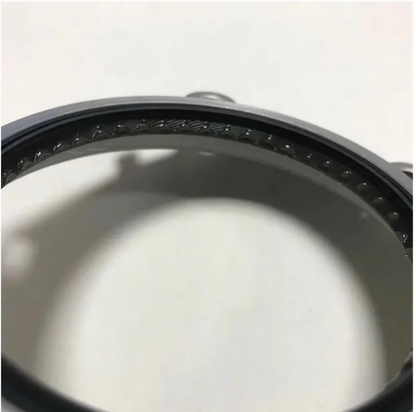
Figure 2.2: A detailed close-up of the sealing lip of the crankshaft rear oil seal. This view highlights the precision-engineered grooves and contours designed to effectively contain engine oil and prevent leaks.
