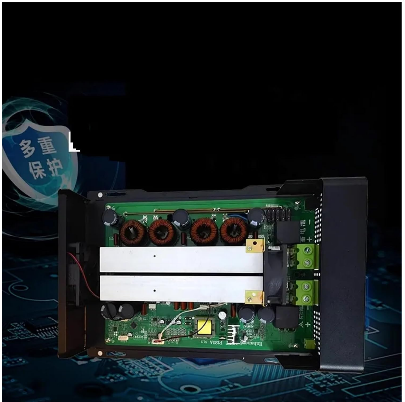
Figure 3.2: Internal view of the DUQTMBDT MPPT Solar Charge Controller, highlighting the power conversion components and circuit board layout.
