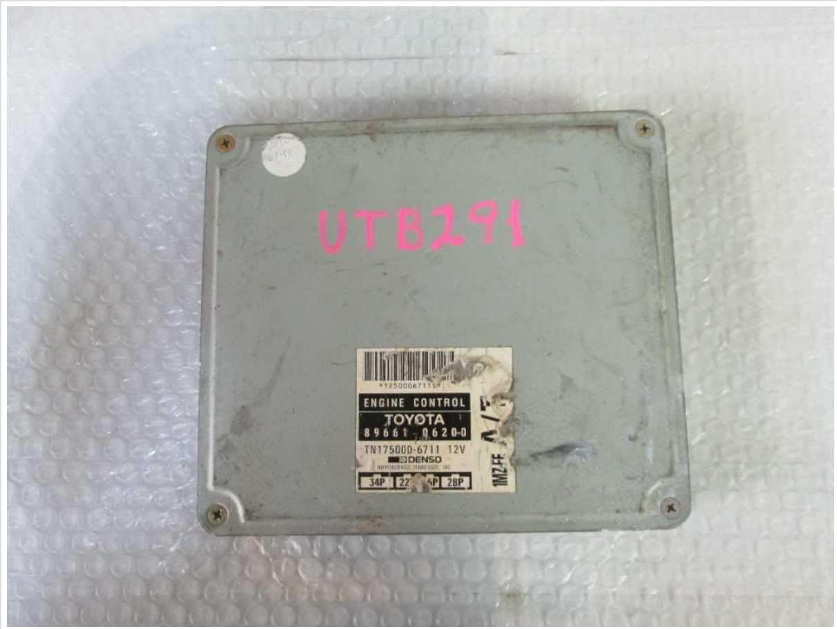
Figure 1: Overall view of the Generic 1995 Toyota Camry Engine ECM Control Module (Part Number 89661-06200).
