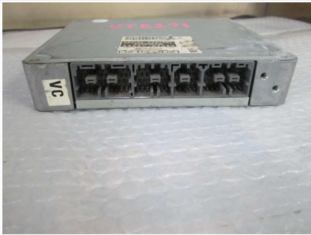
Figure 3: View of the ECM's connector ports, where the vehicle's wiring harness attaches.
