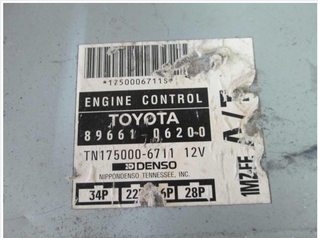
Figure 2: Detailed view of the ECM label, showing the Toyota part number 89661-06200 and DENSO manufacturer information.
