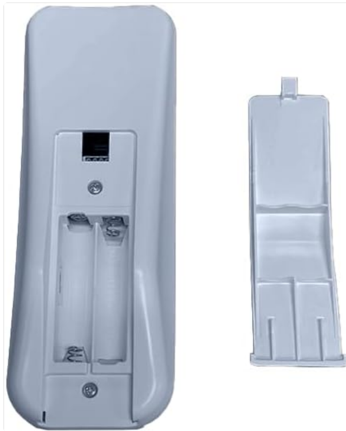
Figure 1: Back of the HJH103 remote with the battery compartment open, showing two AA battery slots.
