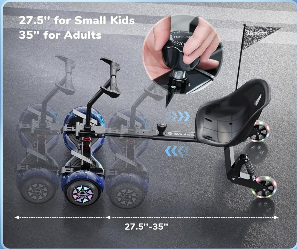
Image 4.4: Demonstrating the adjustable length feature of the attachment.
