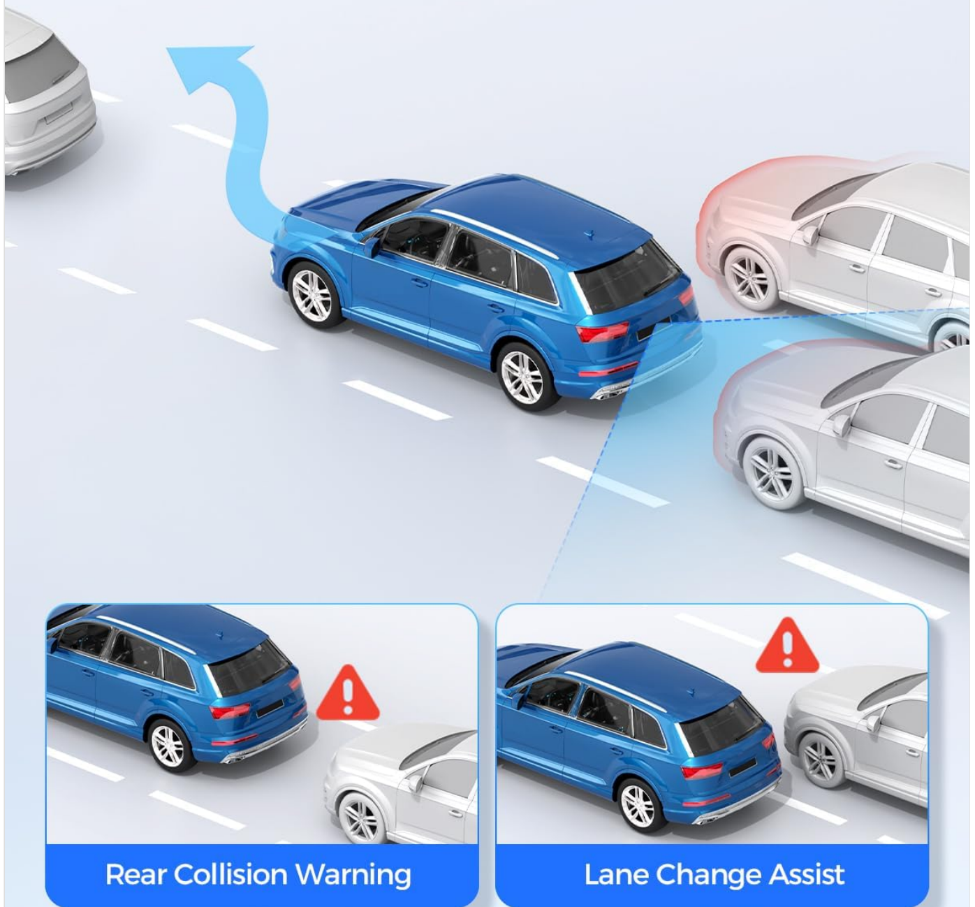
Figure 5.2: Depiction of the Blind Spot Detection (BSD) and Lane Change Assist (LCA) functionalities, showing how the system identifies and warns of vehicles in blind spots.
