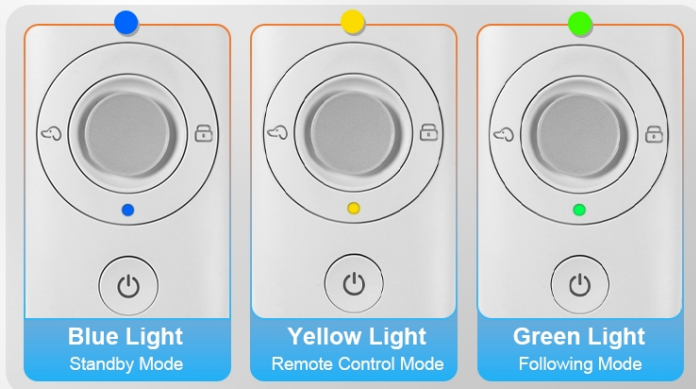
Figure 4.3: The remote control unit, indicating different operational modes via LED lights.
