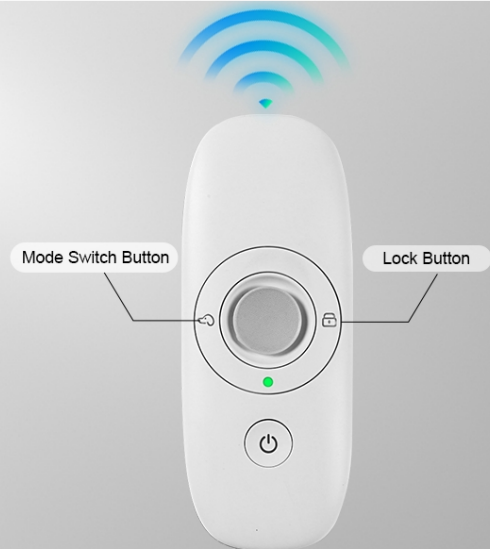
Figure 4.3: The remote control unit, indicating different operational modes via LED lights.
