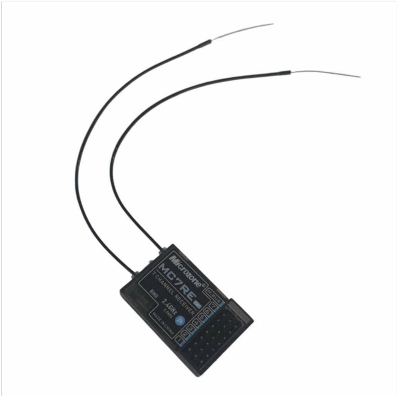
Image 1.1: Overview of the Generic MC7RE V2 7-Channel S-FHSS Receiver, showing its compact design and dual antennas.
