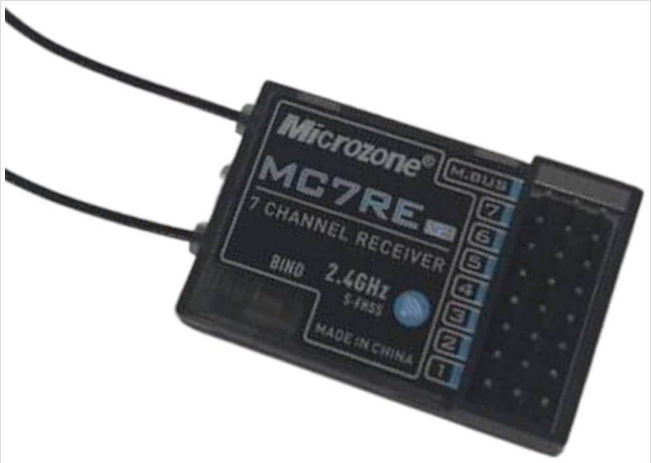
Image 2.1: Close-up view of the MC7RE V2 receiver, highlighting the 'BIND' button and channel ports 1-7, along with the M.BUS port.
