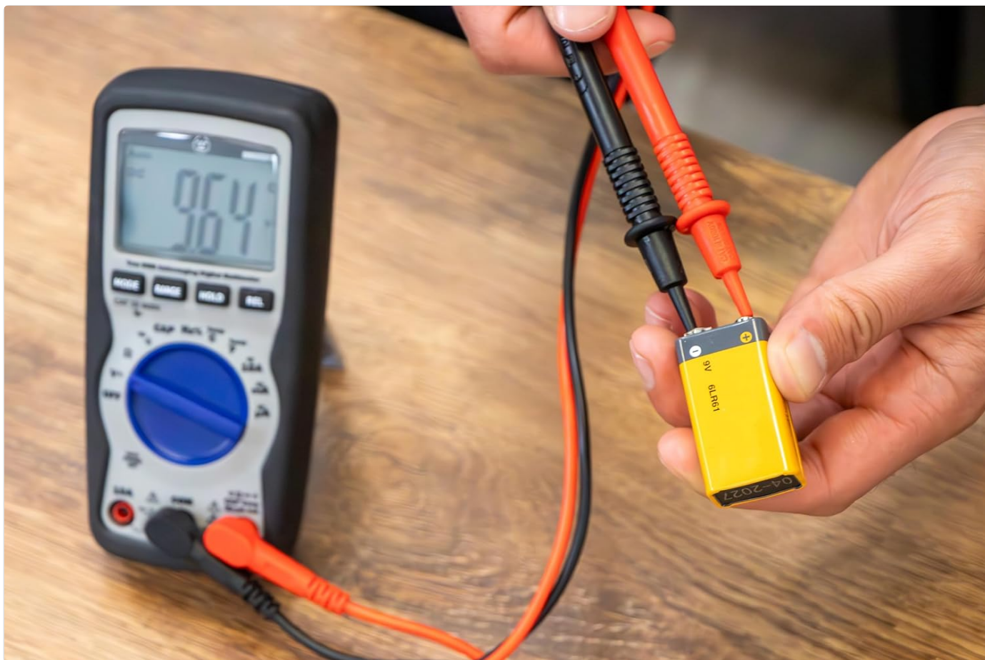
Image: A user connecting a 9V battery to the multimeter's test leads to check its voltage, demonstrating battery handling.
