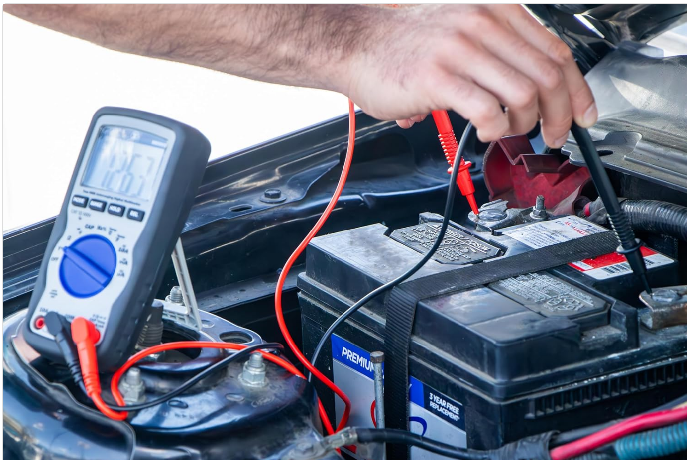
Image: A user measuring DC voltage from a car battery, highlighting the multimeter's utility for automotive applications.
