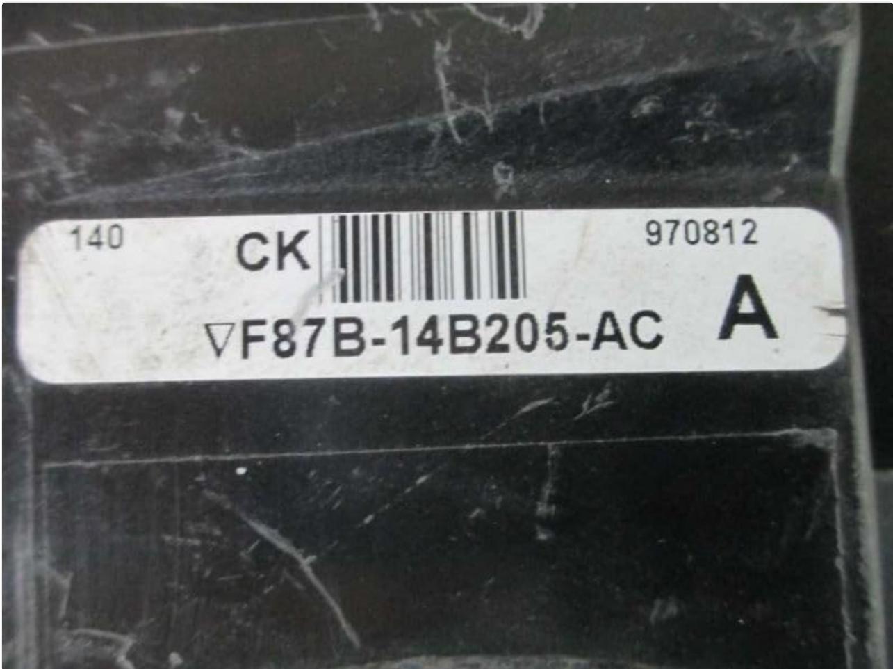
Figure 2: Close-up view of the module's identification label. This image clearly displays the part number F87B-14B205-AC, which is crucial for compatibility verification.
