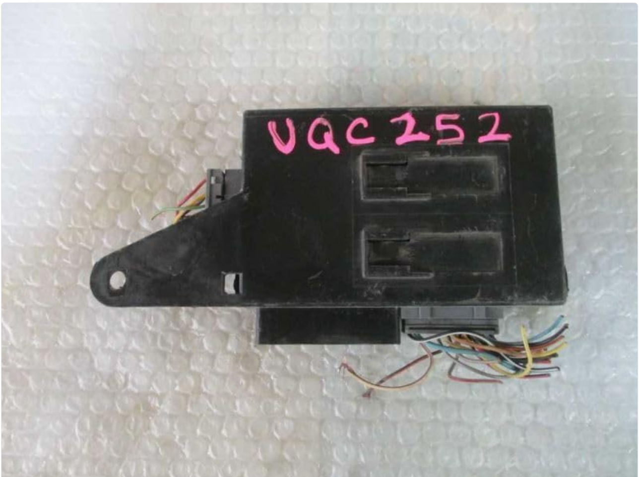
Figure 1: Top view of the Multifunction GEM Control Module. This image shows the main body of the module with visible connectors and the stock number 'UQC 252' marked on it.
