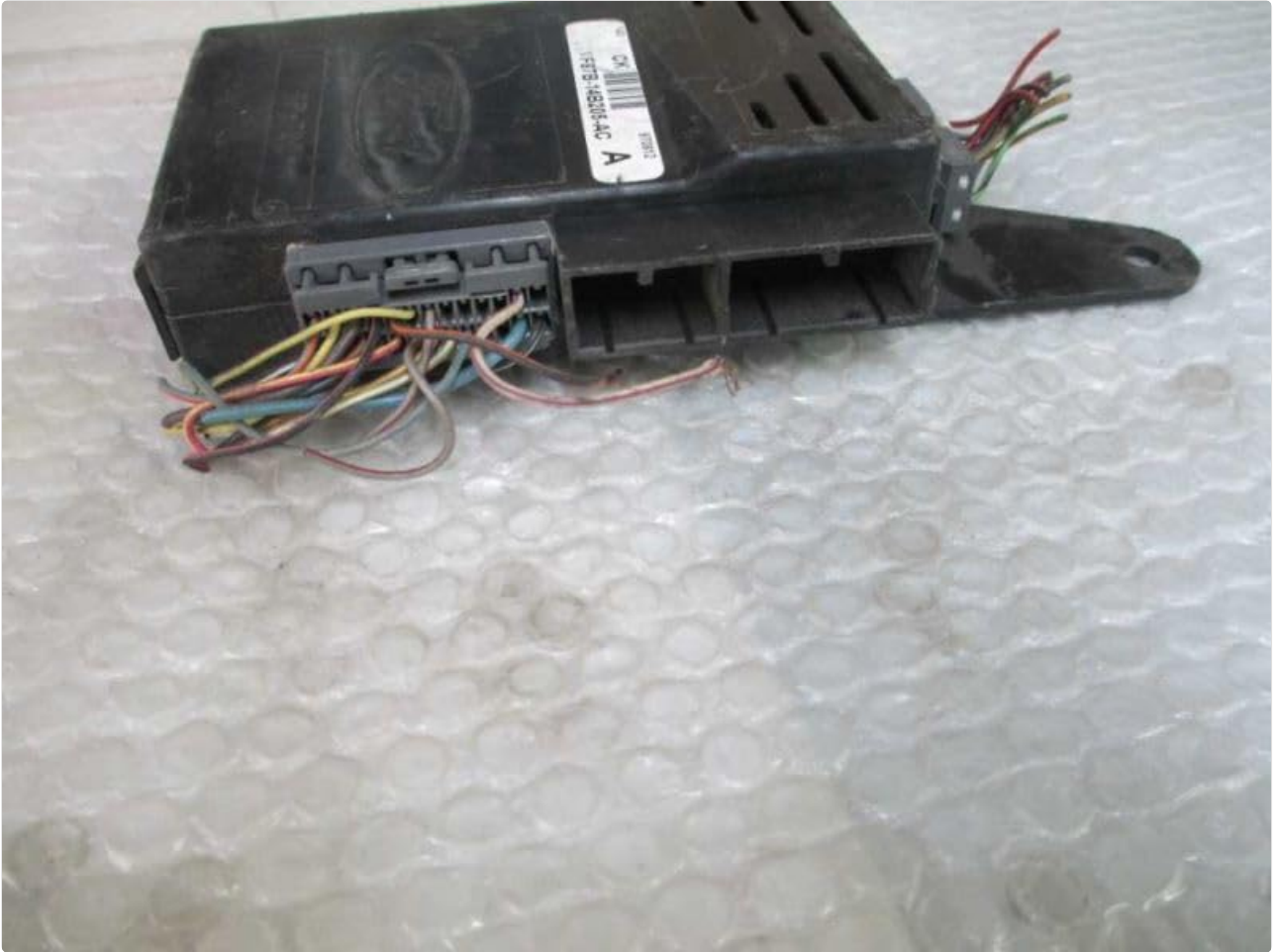
Figure 3: Side view of the module displaying its various electrical connectors. These connectors must be properly aligned and secured during installation.
