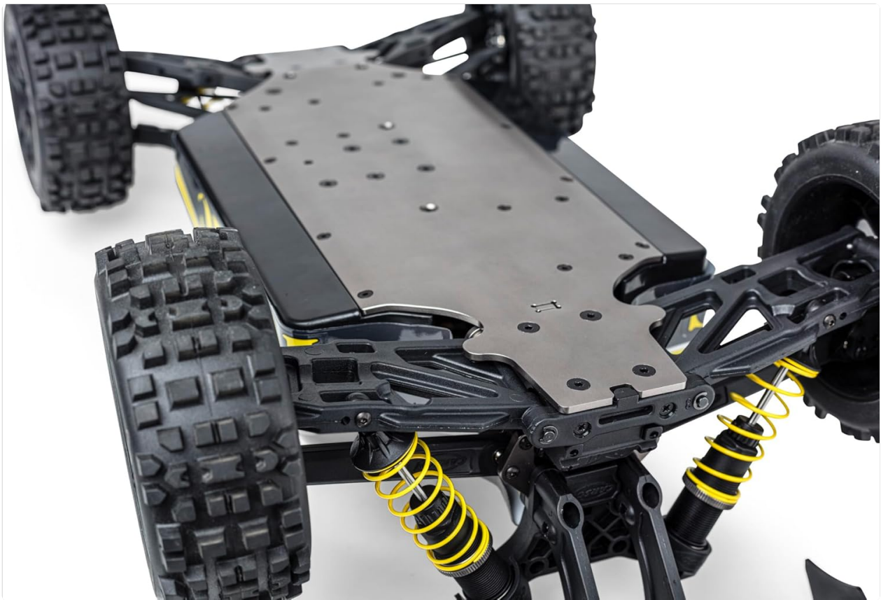
Image 5.1: The robust aluminum chassis of the Akuma Buggy, visible from below, showing the durable construction and suspension system.
