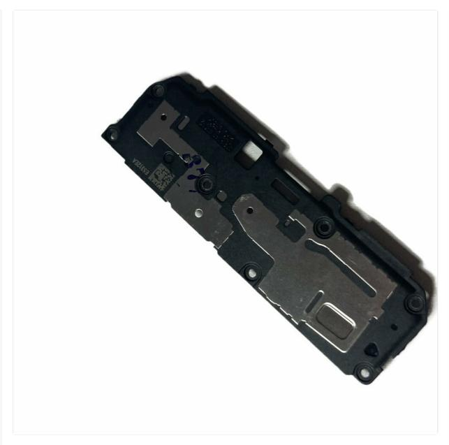
**Figure 2.2:** Rear view of the OEM Loud Speaker Loudspeaker module. This image illustrates the reverse side of the speaker, highlighting its structural backing and mounting points.
