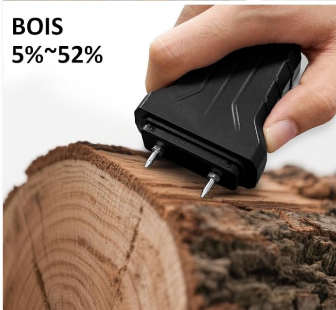
Image 4: Illustration of the measurement depth for the spherical probe and examples of the pin probe measuring moisture in wood and building materials.
