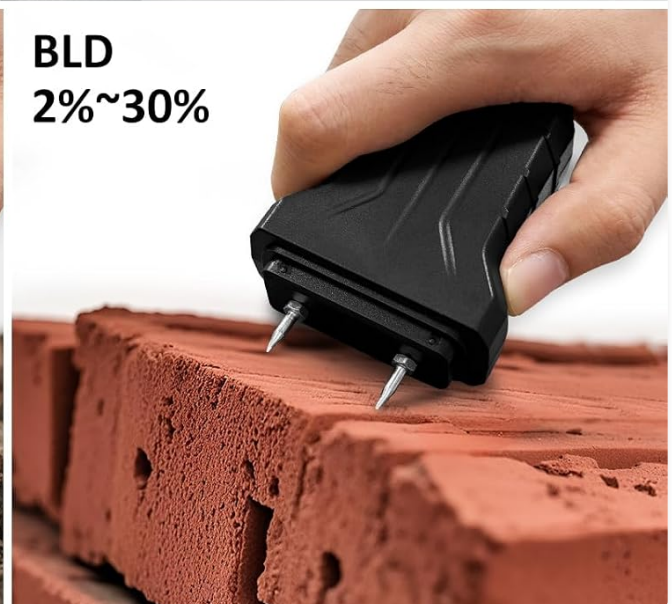
Image 4: Illustration of the measurement depth for the spherical probe and examples of the pin probe measuring moisture in wood and building materials.
