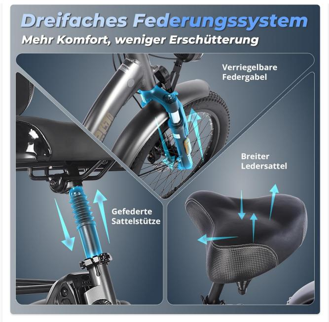
This image details the triple suspension system designed for enhanced comfort. It shows the lockable front suspension fork and the spring-loaded seat post, which work together with the wide leather saddle to absorb shocks and provide a smoother ride.
