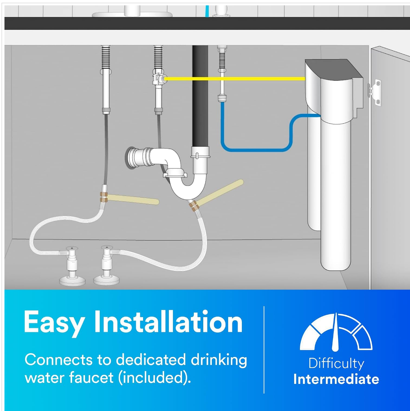
Figure 4: Easy Installation Diagram. This diagram shows a typical under-sink installation setup, illustrating how the filter system integrates with existing plumbing to provide filtered water to a dedicated faucet.
