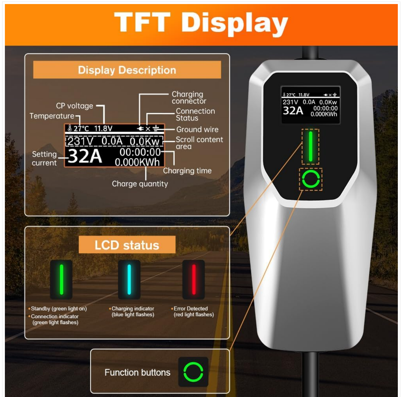
Figure 4.1: Control Box Display Details. This image illustrates the various elements of the charger's LCD screen, including temperature, CP voltage, charging connector, connection status, ground wire status, real-time current, voltage, power, charging time, and charge quantity. It also shows the LED status indicators: green for standby/connection, blue for charging, and red for error detection.
