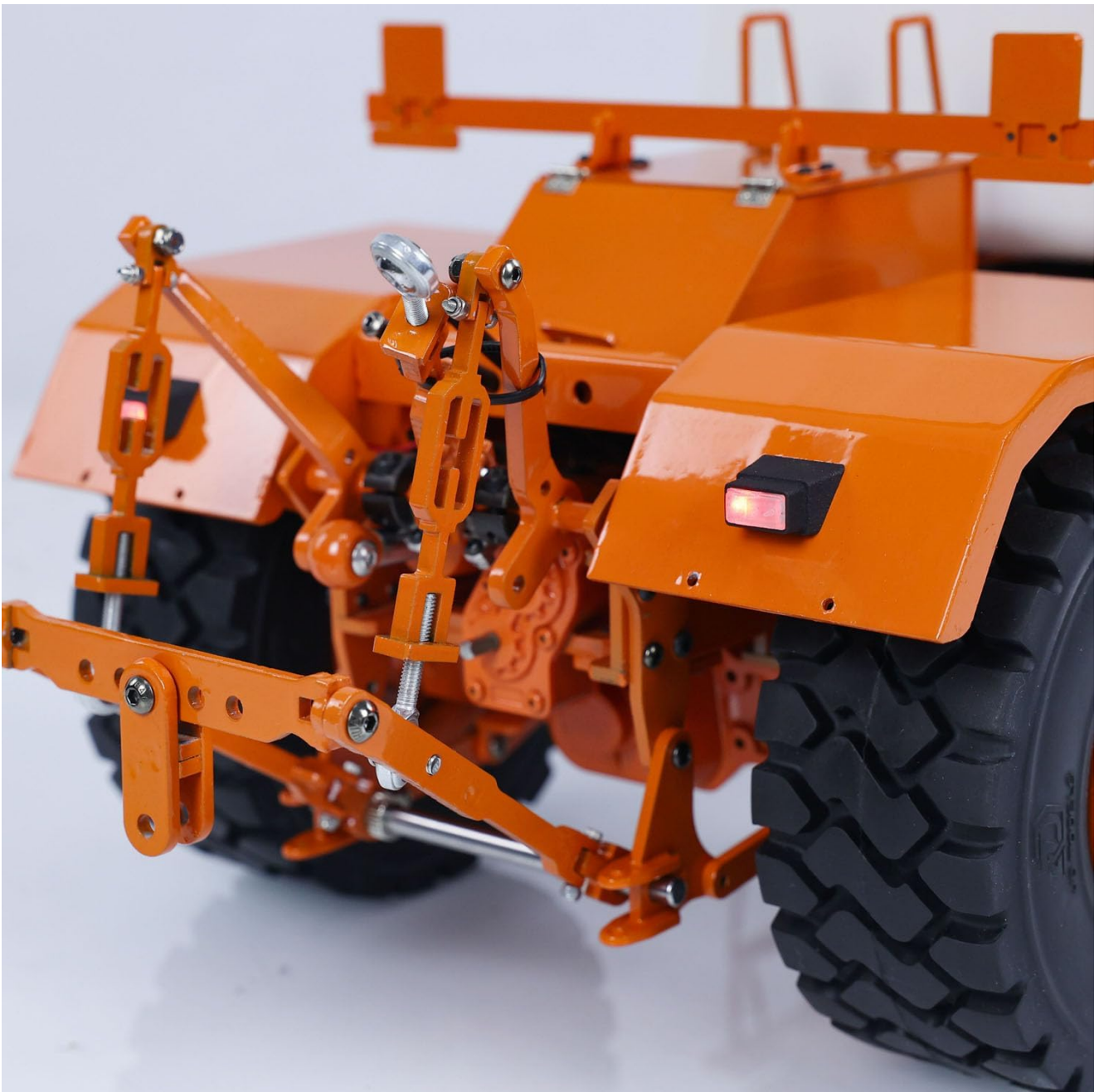
Figure 6: Detail of the rear hitch and suspension system.
