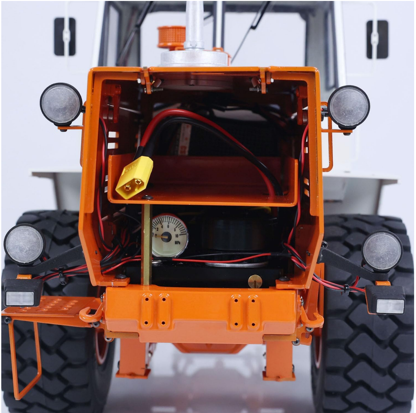
Figure 3: Front compartment with battery connection point.
