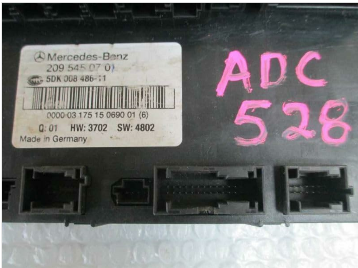
Figure 2.2: Close-up view of the product label. The label clearly shows the Mercedes-Benz branding, part number 209 545 07 01, and additional manufacturing details including "Made in Germany" and internal codes like 0000-03 175 15 0690 01 (6). The handwritten 'ADC 528' is an inventory identifier.
