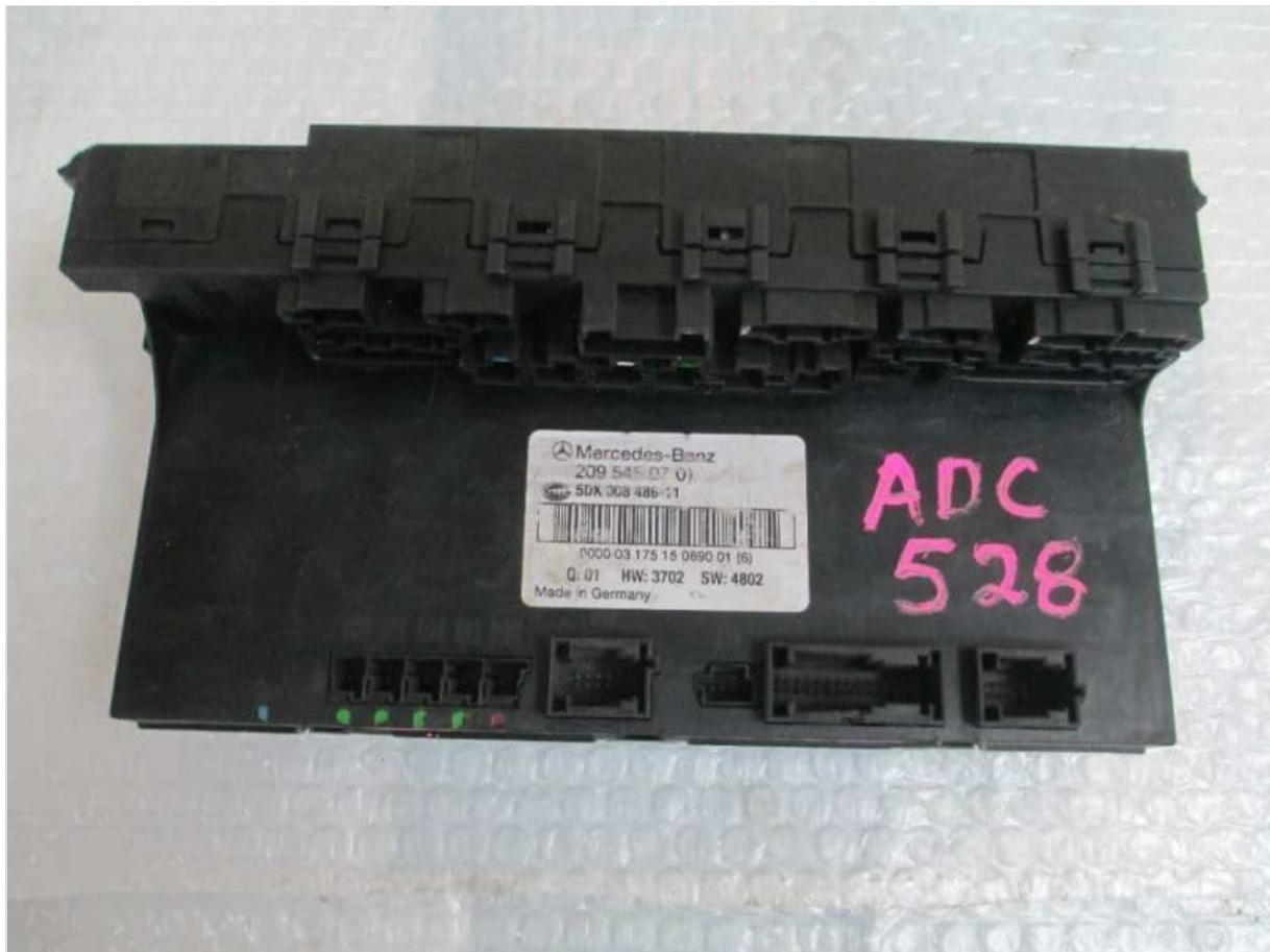
Figure 2.1: Top view of the Mercedes-Benz W209 Rear Trunk SAM Fuse Relay Box. This image displays the overall structure of the unit, including various connector ports and the main label.
