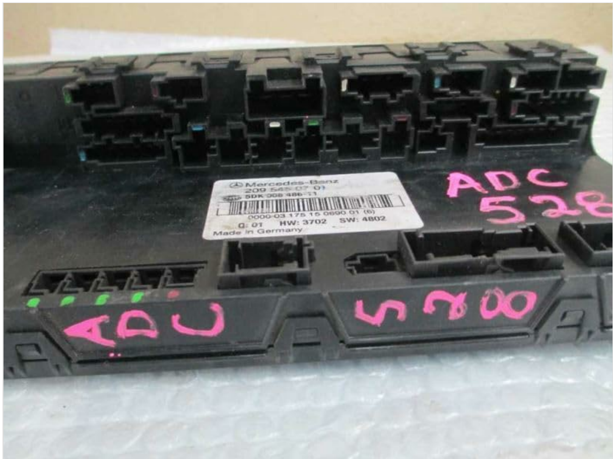
Figure 4.1: Angled view of the SAM unit, highlighting the various electrical connectors and their arrangement. Proper connection of these is crucial during installation.
