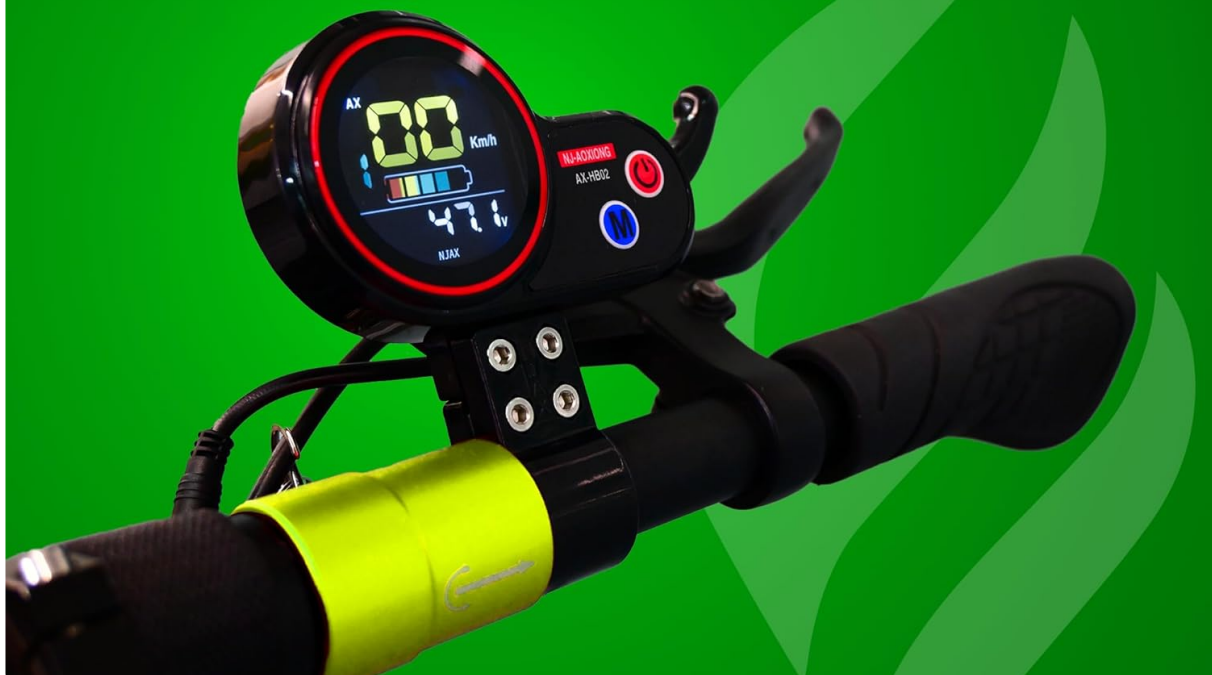
Image 5.2: Close-up view of the Evobike M1's LED display, showing speedometer, distance, battery, and light controls.
