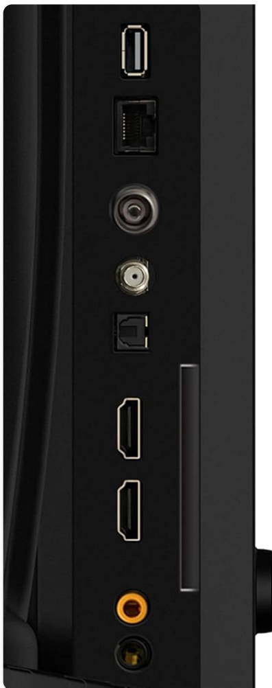
Image: Close-up of the TCL 32V4C TV's connectivity ports, including HDMI, USB, Optical, Cable, Satellite, AV Input, Headphone, and CI Slot.
