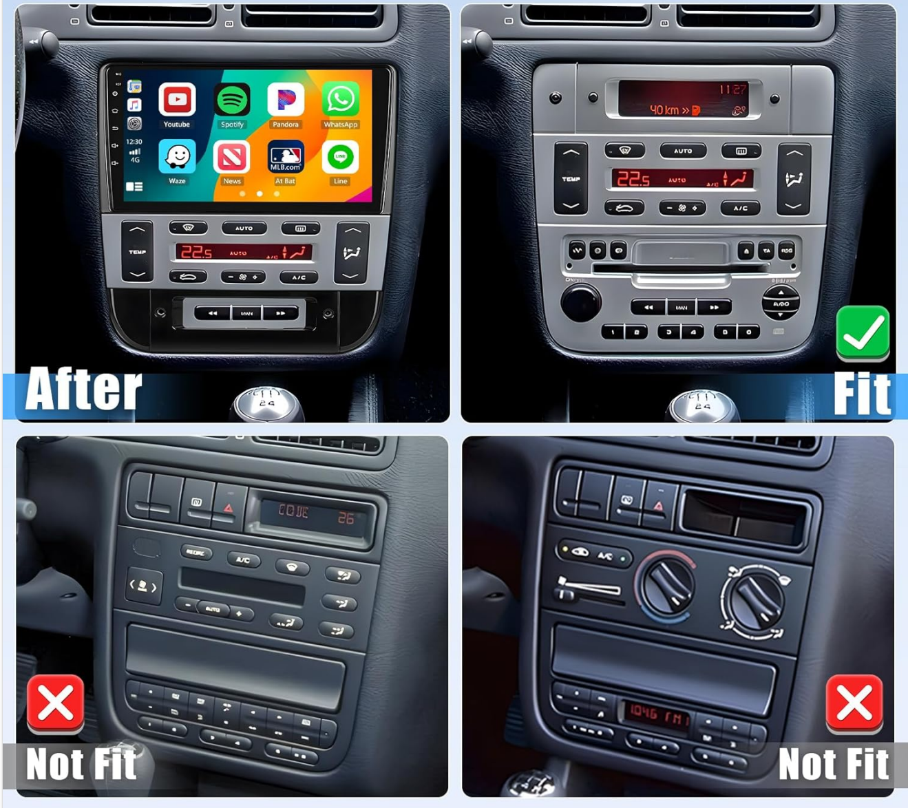
Image 2.2: Illustration showing compatible (top right) and incompatible (bottom left and right) dashboard configurations for the Peugeot 406.
