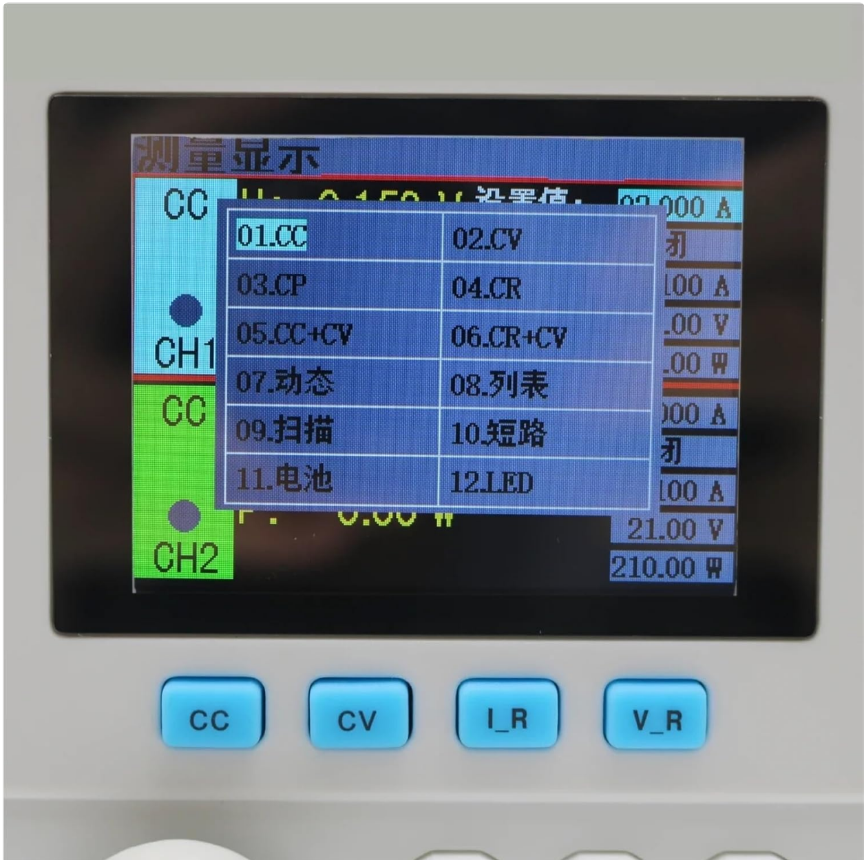
Figure 3.2: Display showing the selection menu for various measurement modes, including CC, CV, CR, CP, and specialized tests.
