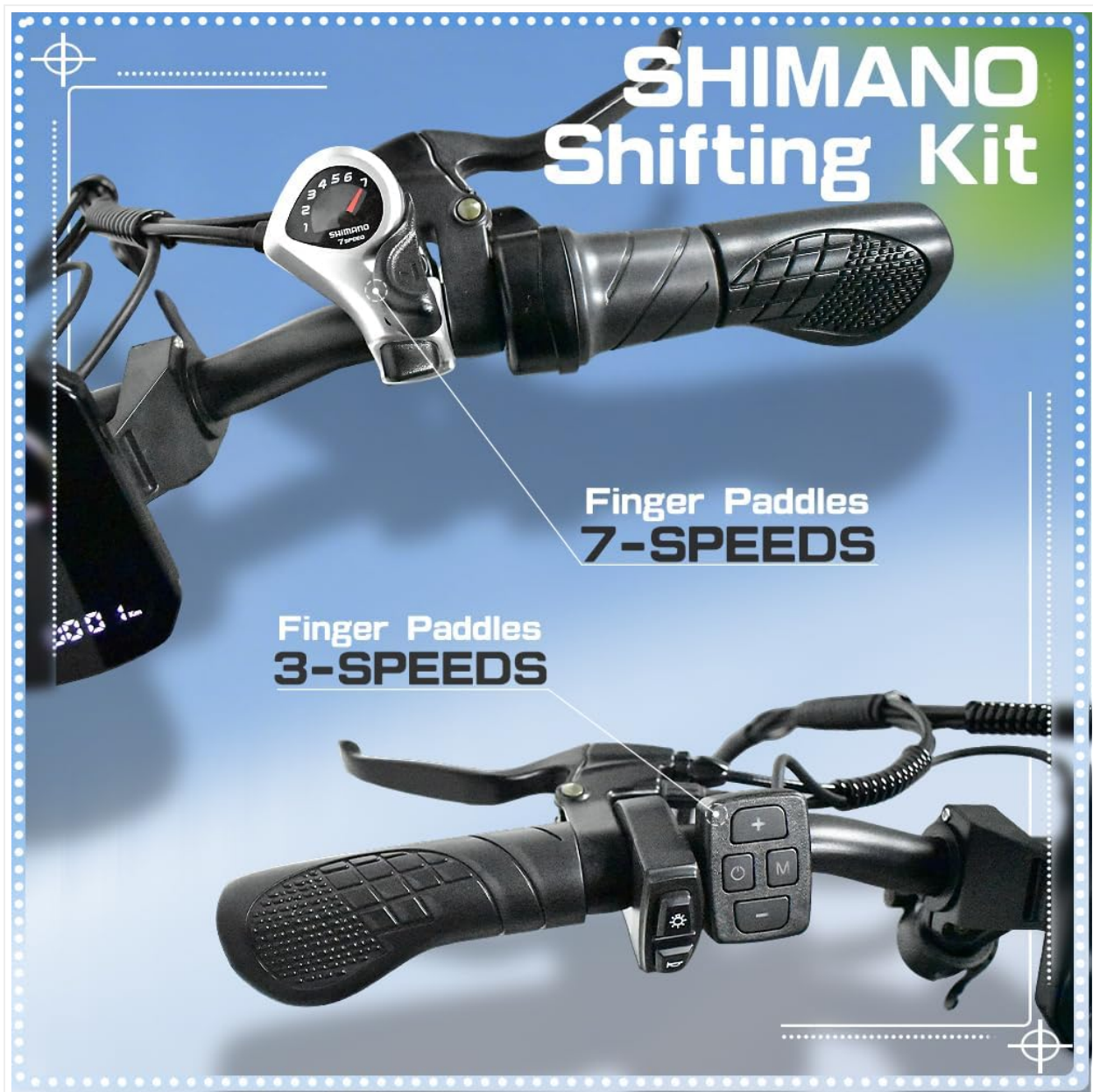
Close-up of the SHIMANO shifting kit, illustrating the 7-speed finger paddles for gear changes.
