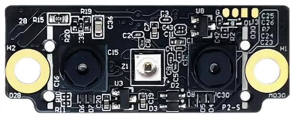
Figure 1: Bloepum FM225 3D Face Recognition Module. This image displays the compact circuit board of the FM225 module, featuring two camera lenses and an infrared LED in the center, along with various electronic components.
