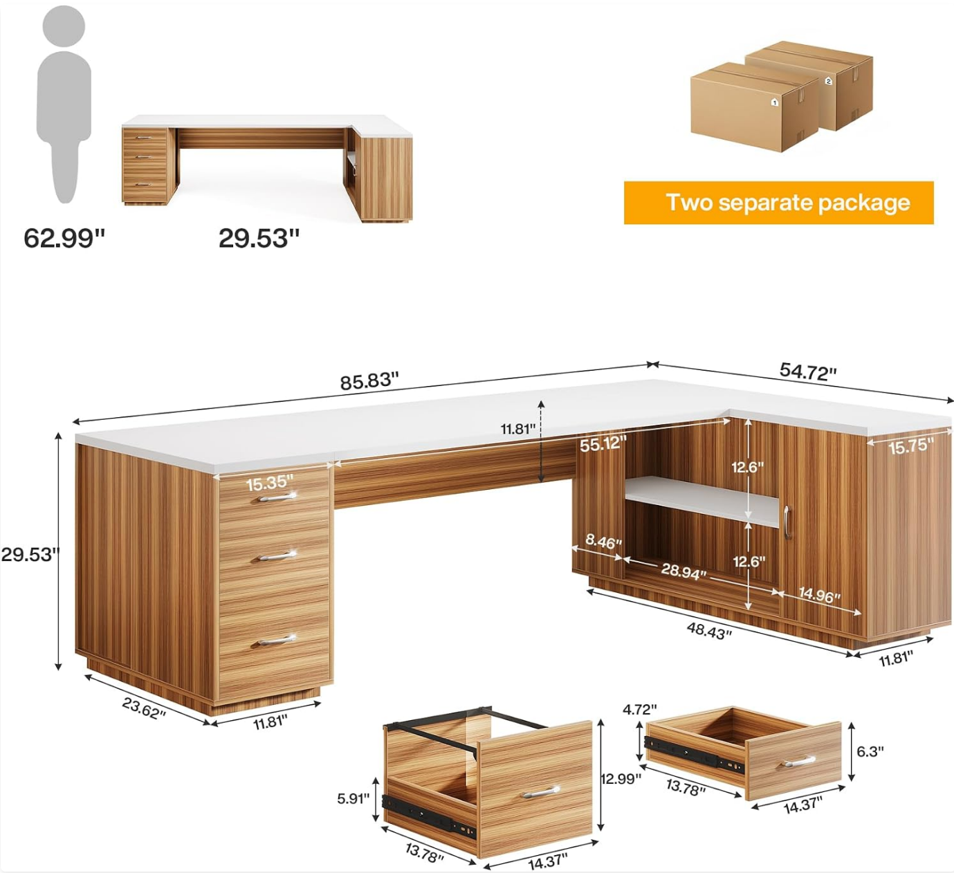
Detailed dimensions of the L-shaped desk, including measurements for the desktop, drawers, and storage compartments.
